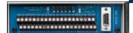
The Cell682 has 8 Dry Contact inputs that can be used to monitor Normally Open (N.O.) or Normally Closed (N.C.) sensors and 6 Analog inputs that can be used to monitor 2.8K or 10K Thermistors (temperature) or 4-20mA transducers.
