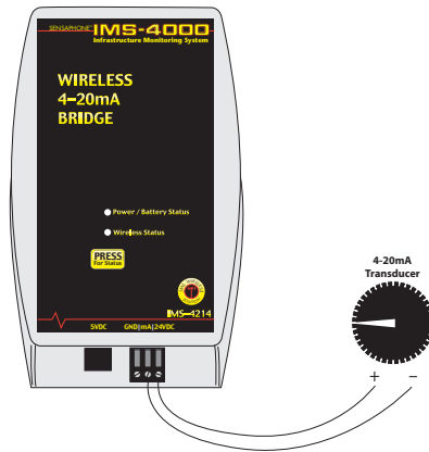
4-20mA Transducer using 24VDC power supply
